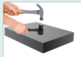
hammer impact to apply test force
